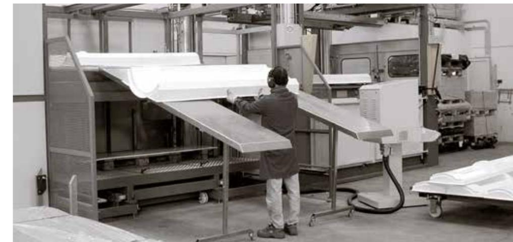
Thermoforming plant for acrylic materials.
