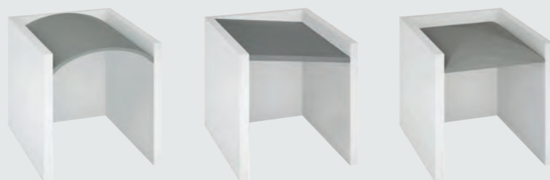
Volta a botte Barrel vaulted ceiling Voute en berceau
