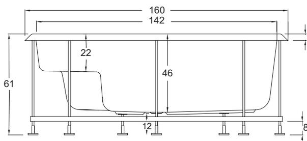
If the bath is recessed the masonry cannot reenter more than the masonry must fall back to the outer edge of 2 cm. An inspection panel and air intake must be installed.
