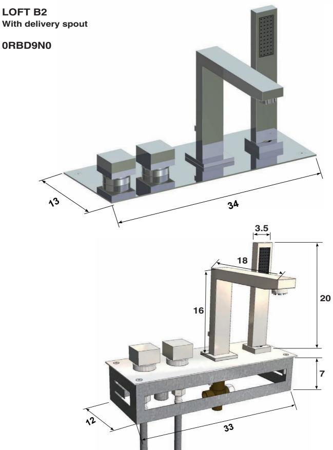
The overall dimensions are given in centimetres. Actual dimensions can vary by  $\pm$  1 cm.
