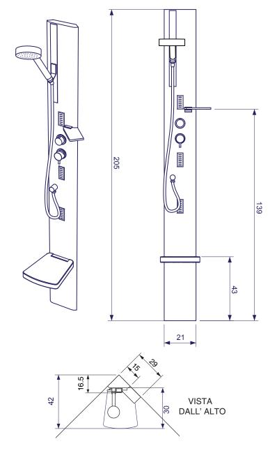
The overall dimensions are given in centimetres. Actual dimensions can vary by  $\pm 0.5$  cm.
