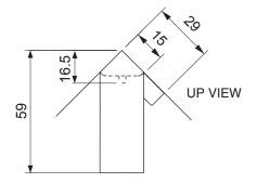
The overall dimensions are given in centimetres. Actual dimensions can vary by  $\pm 0.5$  cm.
