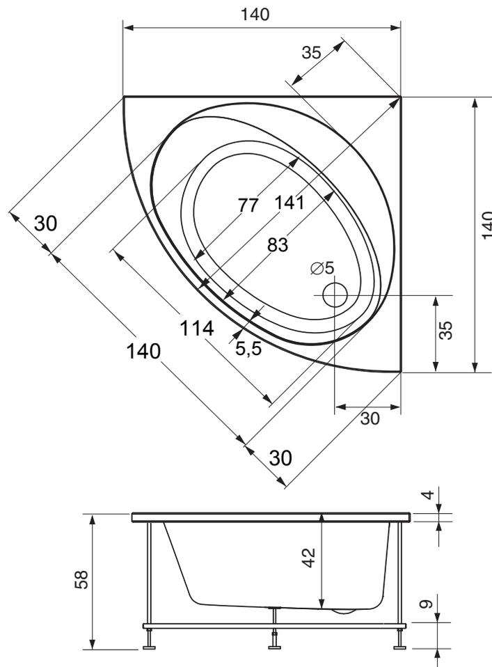
If the tub is installed flush, the wall can not fall from the outer edge more than 1 cm. Provide for the inspection panel and snorkel. In tubs Whirlpool and Whirlpool airpool the pipes are at the outer edge of the tub.
