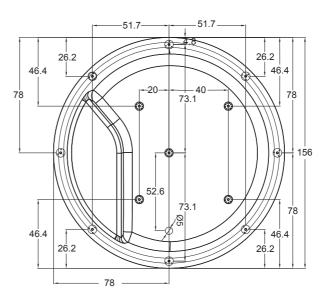
The overall dimensions are given in centimetres. Actual dimensions can vary by  $\pm$  1 cm.
