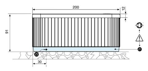
make a hole (with dimensions suitable for passing the power cable through it) in one of the 4 sides of area **Z1**.
